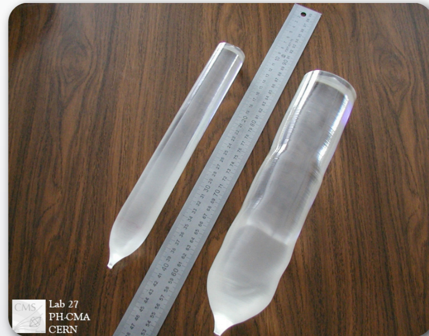
PbWO 4 : used for electromagnetic calorimeter in CMS
