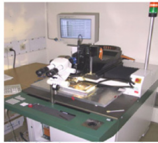
Wirebonding of 900 modules
