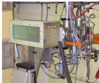
Test of radiation hardness at cyclotron
