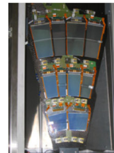
IEKP: Construction of 102 Petals for tracker (30%)
