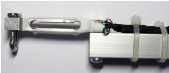
NTC-Widerstand  $R_{25} = 10 \text{ k}\Omega$
