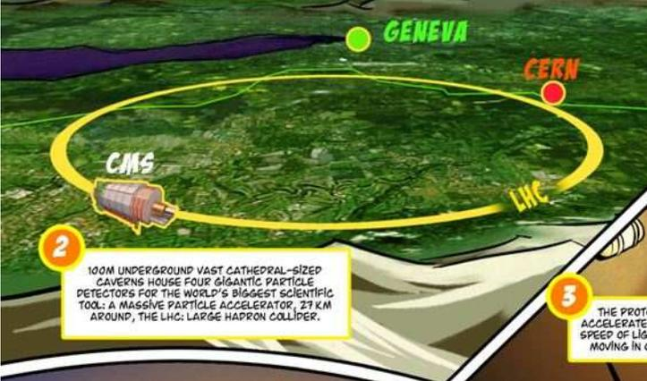
**2** 100M UNDERGROUND VAST CATHEDRAL-SIZED CAVERNS HOUSE FOUR GIANT PARTICLE DETECTORS FOR THE WORLD'S BIGGEST SCIENTIFIC TOOL: A MASSIVE PARTICLE ACCELERATOR, 27 KM AROUND, THE LHC: LARGE HADRON COLLIDER.
