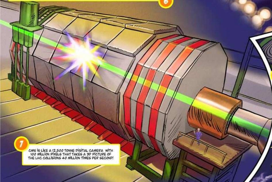
**7** CMS IS LIKE A 12,500 TONNE DIGITAL CAMERA WITH 100 MILLION PIXELS THAT TAKES A 3D PICTURE OF THE LHC COLLISIONS 40 MILLION TIMES PER SECOND!
