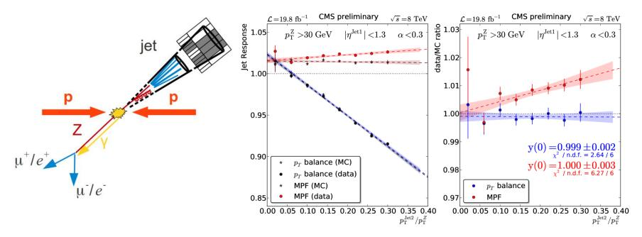
$$R_{balance} = \frac{p_{T}^{jet}}{p_{T}^{\gamma/Z}} \text{ and } R_{MPF} = 1 + \frac{\vec{E}_{T}^{miss} \cdot \vec{p}_{T}^{\gamma/Z}}{\left(p_{T}^{\gamma/Z}\right)^{2}}$$
