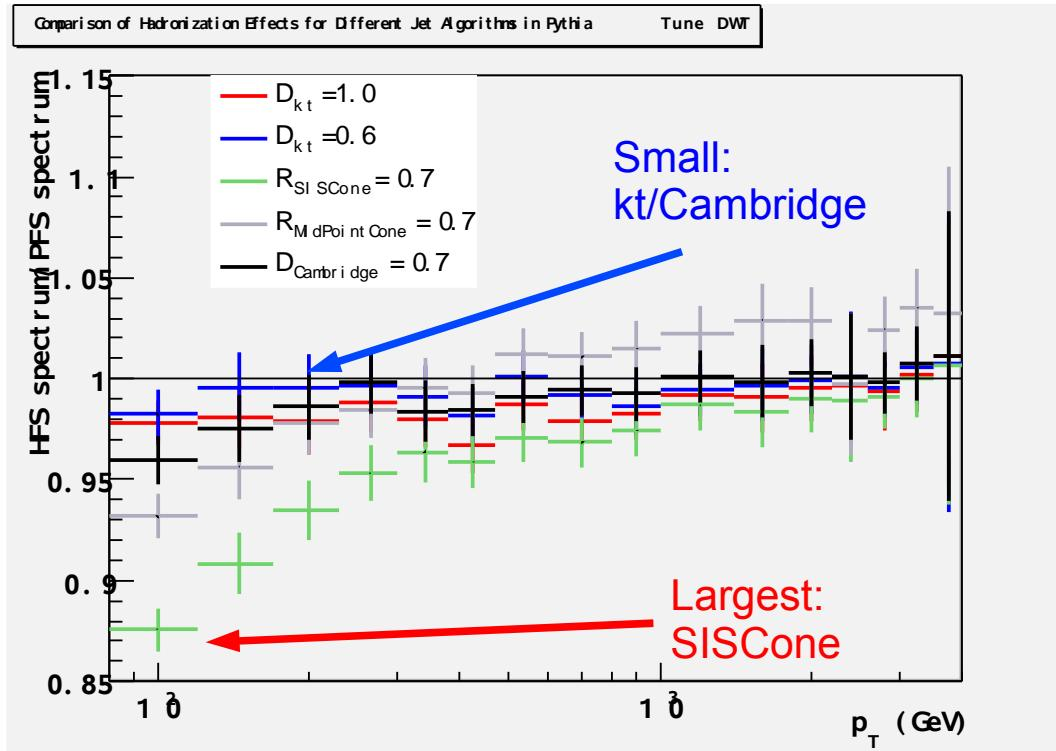
Dependence on jet algorithms of  $p_t$  balance in  $Z + \text{jet}$  events (MC)
