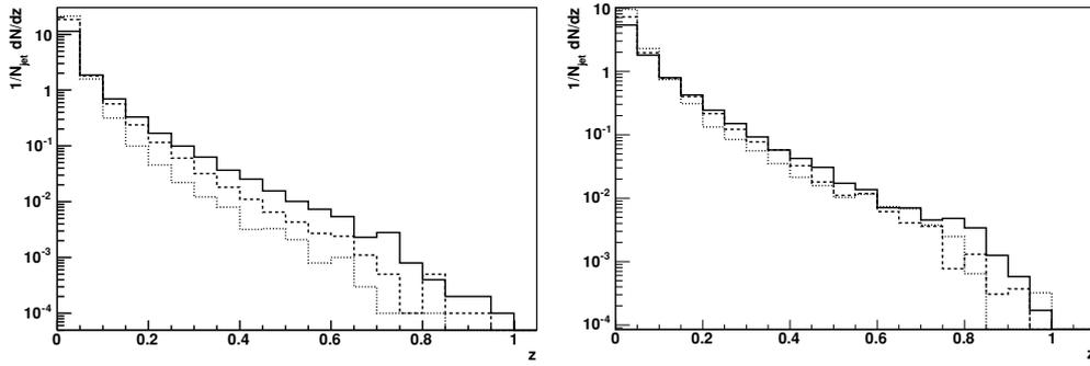
**Figure 2.** Fragmentation function for 100 GeV jets unquenched (solid), quenched with AliQuench (dashed) and PYQUENCH (dotted). The left distribution is obtained without the inclusion of detector effects and  $R < 1$ . The right plot includes the finite jet resolution and a systematic underestimation of the parton energy as described in the text.
