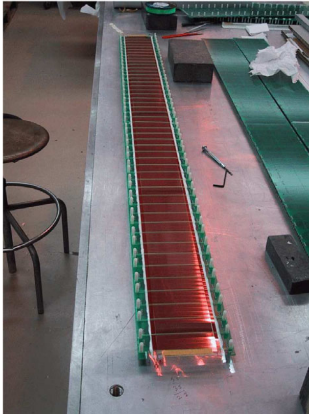
Figure 3.19. Photograph of an MRPC strip during construction.
