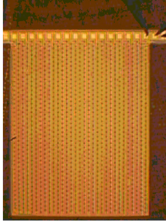
Figure 5.24: Pure 3D detector with microstrip readout configuration. The electrodes and the aluminium strips, which tie the rows of p^+ and n^+ electrodes, are clearly visible. The p^+ strips end at the bonding pads (top)
