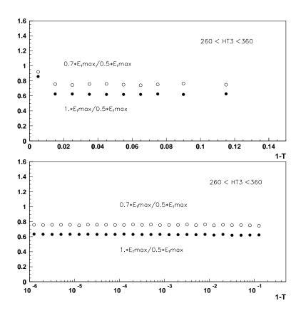
Figure 8.20: Dependence of Jetrad  $T_2^t$  distributions on the renormalization scale for the second bin of HT3. The open circles correspond to the ratio of  $0.7*E_Tmax/0.5*E_Tmax$  and the full ones to  $1*E_Tmax/0.5*E_Tmax$ .
