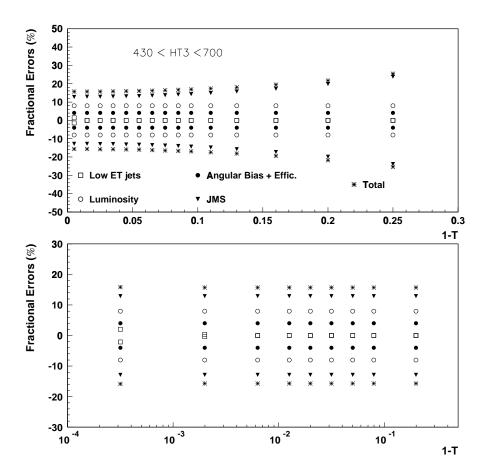
Figure 8.4: Fractional experimental uncertainties as a function of  $1-T_2^t$  in linear and logarithmic scale. The total errors correspond to the quadrature sum of each of the contributions shown in the plots (it does not include the contribution from the error on the unsmearing factors).
