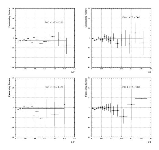
Figure 7.15: Unsmearing factors as a function of 1-T. The bars are the statistical errors. The correction has been extracted from the points up to 1-T=0.04 (this is the region where most of the statistics resides). From there, in order to smooth out the curve, the points are fitted with a constant function.
