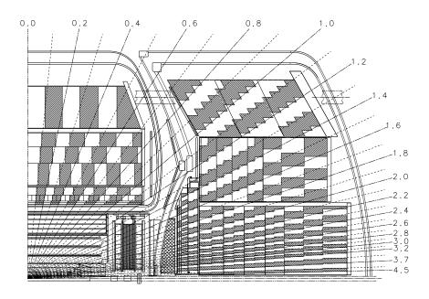
Figure 2.6: Side view of calorimeter towers.
