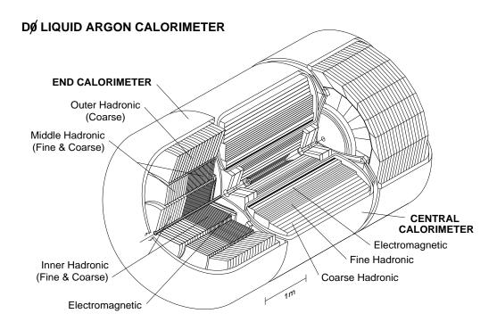
Figure 2.4: General view of the DØ calorimeters.
