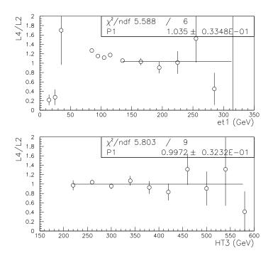
Figure B.2: Top: Ratio between the leading jet  $E_T$  spectra for two subsamples of  $Jet\_50$ . Bottom: Ratio between the HT3 spectra for the same subsamples, the distributions have been normalized to account for inaccuracies on PDB results.
