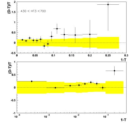
Figure 8.28: Data comparison with NLO 3 jets NLOJET++ prediction. The bars correspond to the statistical errors while the bands are the systematic ones.
