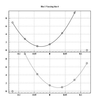
Figure 7.17:  $\chi^2$  difference between smeared distributions for two different ansatz distributions: the nominal (shown in Figure 7.14) and the same one with 4% events added (subtracted) in bin 4 for the top (bottom) plot. The abscissa corresponds to the fractional variation of events in bin 1. This example shows negative correlation between the two bins. The plot corresponds to N-paraboloid fit in equation 7.2.
