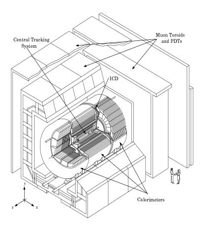
Figure 2.2: A general view of the Run I DØ detector
