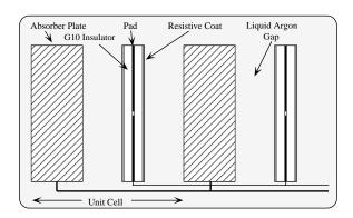
Figure 2.5: Schematic view of a calorimeter cell.
