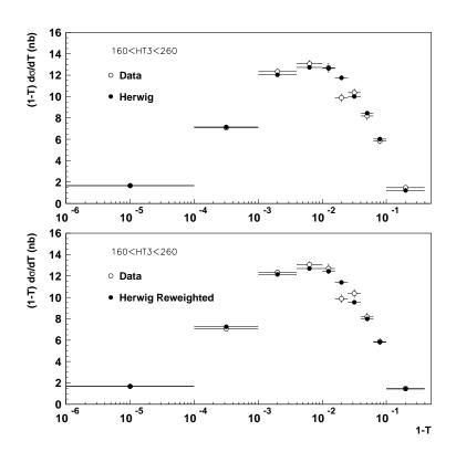
Figure 7.14: Top: Data comparison with the Herwig particle level distribution smeared by  $E_T$ ,  $\eta$  and  $\phi$  resolutions for the lowest HT3 bin. Bottom: MC events have been reweighted in order to make the smeared distribution agree with data.
