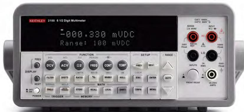
The Keithley Instruments Model 2100 is a rugged and versatile 6 1/2-digit resolution digital multimeter. It has 0.003% one-year basic DC voltage accuracy at 10V range and 0.005% one-year basic resistance accuracy at 10k $\Omega$  range. At 6 1/2 digits, the multimeter delivers 50 triggered RDGS/sec via the USB remote interface. At the fast 4 1/2-digit setting, it reads over 2000 RDGS/sec into its internal buffer.
