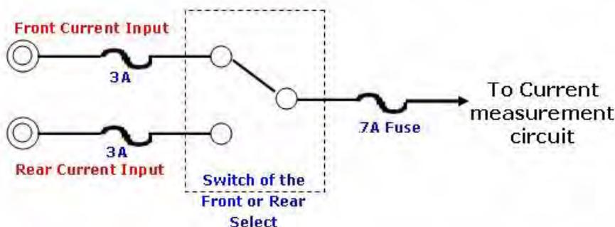
The two main fuses located in the front and rear current input terminals of your Model 2100 are 3A, 250V, 5x20mm fast-acting glass fuses (Keithley Instruments part number FU-99-1). The additional current input fuse is a 7A, 250V, 5x20mm fast-acting ceramic tube fuse. See the following text for instructions on how to replace these fuses if they become damaged.
