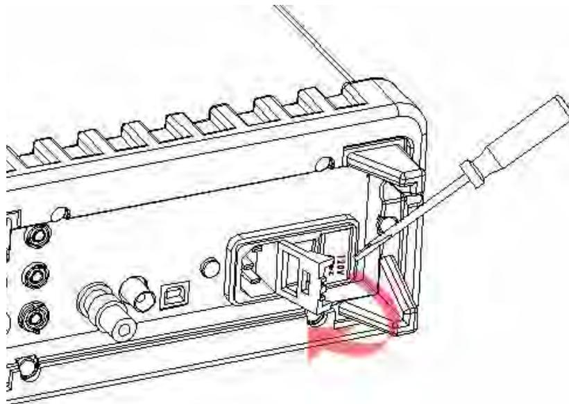
**Step 3: Remove the red voltage setting selector**
