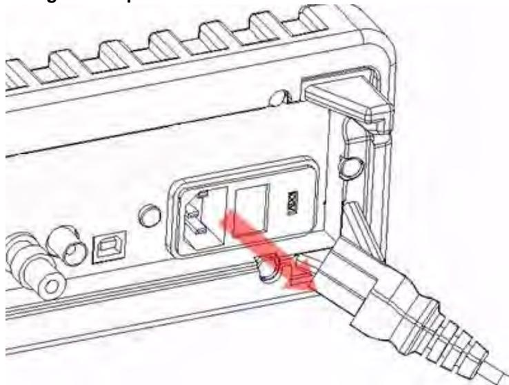
**Step 2: Release the current input terminal fuse holder**
