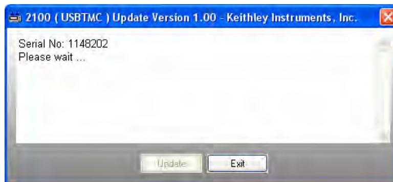
6. Once installation of the DSP firmware update file is complete, you will be prompted to restart your Model 2100 to continue the update (see [Figure 4-38](#)). Power the Model 2100 off, and then power it on again.
