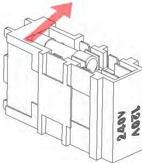
**Step 5: Replace the power line fuse**
