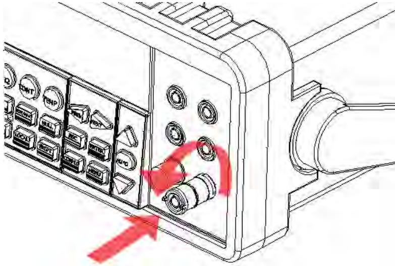
**WARNING** Before reconnecting the power line cord to your multimeter, make sure that the power switch is in the "POWER OFF" position.
