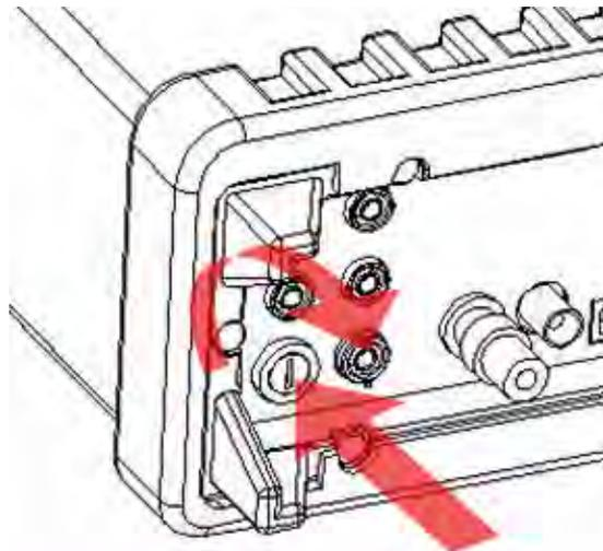
**WARNING** Before reconnecting the power line cord to your multimeter, ensure that the power switch is in the "POWER OFF" position.
