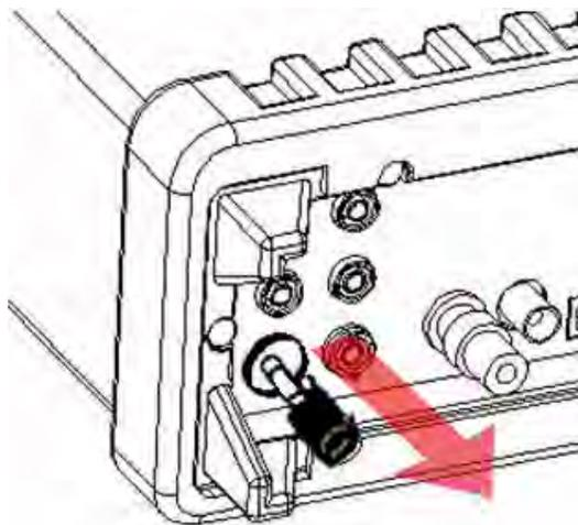
**Step 4: Remove and replace the damaged fuse**
