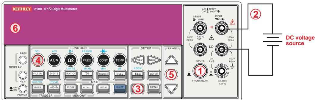
Input resistance = 10M $\Omega$  on 1000V and 100V ranges:
