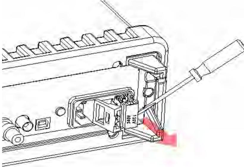
**Step 4: Remove the damaged power line fuse**
