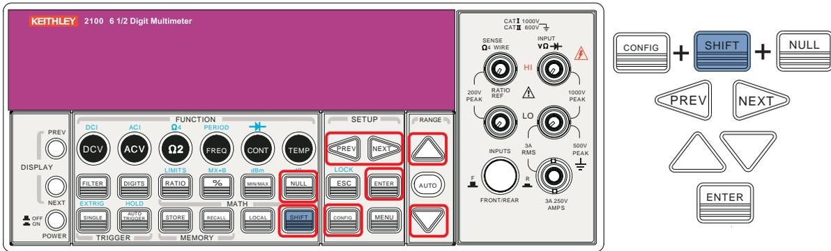
**To make a dB measurement from the front panel:**
