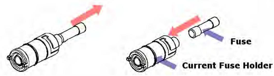
**Step 5: Reinsert and secure the 7A current input terminal fuse holder**
